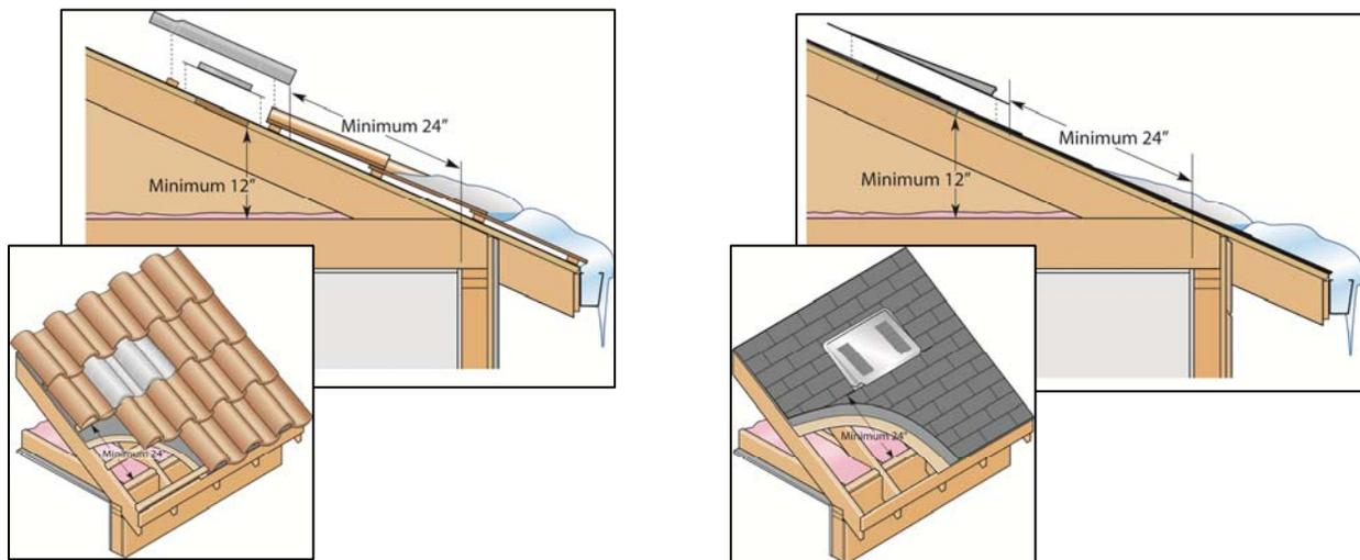
Generally, best roofing and construction practices will dictate the construction methods in any given area. Please defer to local best practices when designing your attic ventilation plan as well as the manufacturer recommendations and installation instructions when installing O'Hagin attic ventilation products with other roofing materials.
