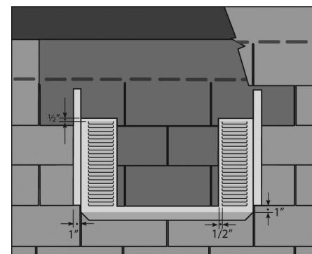
**2. BEGINNING WITH COURSE 1**, align and attach to top of vent as shown using locally-approved peel and stick, two-sided tape, or sealant (Class A where required by code for flame resistance). Repeat with Courses 2 and 3 to complete shingle-over finish method.
