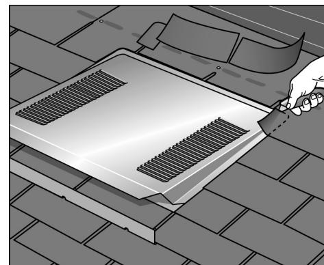
**6. TRIM** roofing material back 1-inch on top and sides of vent cover to allow for proper drainage.
