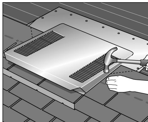
**5. COVER** with roofing material around vent. Based upon local best practices, a 45-degree angle cut may be made on the material terminating at the vent. **See Step 5a. if installing shingle-over finish method.**
