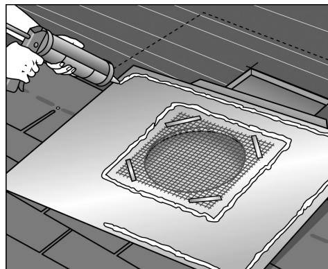
**2. SEAL** using sufficient amount of locally-approved sealant (Class A where required by code for flame resistance) around inner and outer flange.
