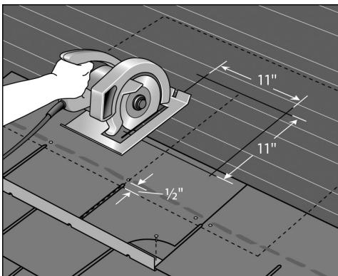
**1. MARK & CUT\*** Align front of vent 1/2-inch below nail line and mark outline of vent for placement later. Mark outline of 11-inch by 11-inch hole. With blade set to thickness of sheathing, cut hole in roof deck.
