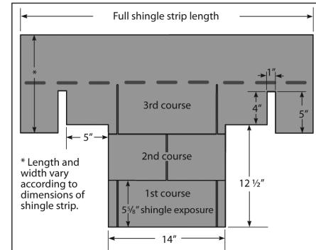
**1. TRIM** two shingle strips to lengths shown for Courses 1 and 2. Using a full length of shingle strip, trim to pattern dimensions shown for Course 3.
