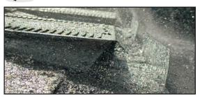
**TESTED** to 140 mph wind-driven rain (category 4 hurricane). **PASSED:** Wind-driven rain tested for 75 feet–five plus stories.
