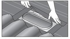
4. FLASH When using peel and stick or membrane and mastic methods, apply bottom strip first, then sides and finally the top strip. For proper drainage around the raised lip of the primary vent (subflashing) hold roofing material back a minimum of one finger width. (See No. 2 in the General Instruction Notes below.)
