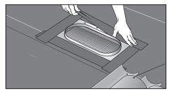
2. SEAL, ATTACH & FLASH subflashing as shown in Steps 2-4 of the High Profile (S) installation instructions. Apply field tile up to the subflashing, nailing the wire into place.
