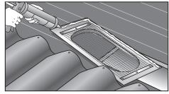
2. SEAL using a sufficient amount of locally-approved sealant around outer flange of primary vent.
