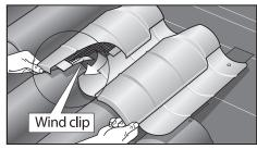
**5. INSTALL** the secondary vent (cover), bending the wind clips tightly under the preceding course of tile, adjusting for head lap.
