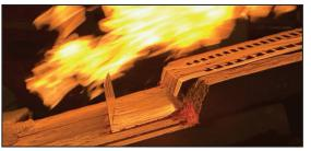
**TESTED** to meet the specific requirements of Chapter 7A of the California Building Code for flame and ember exposure. **PASSED:** NO cotton ignition.
