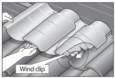
**4. INSTALL** the new secondary vent (cover), bending the wind clips tightly under the preceding course of tile, adjusting for head lap.
