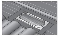
INSPECT existing subflashing to ensure it's been properly installed in accordance with manufacturer's installation instructions (See No. 2 in the General Instruction Notes below).
