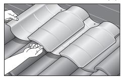
REMOVE surrounding roof tiles, existing secondary vent (cover) and any debris on or near the primary vent (subflashing).
