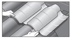
**1. REMOVE** surrounding roof tiles, existing secondary vent (cover) and any debris on or near the primary vent (subflashing).
