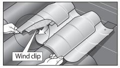
4. INSTALL the new FIRE&ICE® cover, bending the wind clip tightly under the preceding course of tile, adjusting for head lap.
