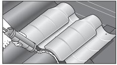
5. SEAL any gaps between FIRE&ICE® cover and surrounding tiles, as well as any fastener penetrations using locally-approved Class A sealant for flame and ember resistance.
