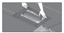
2. SEAL, ATTACH & FLASH as shown in Steps 2-4 of the 1-piece installation instructions. Apply field tile up to the sub flashing, nailing the wire into place.
