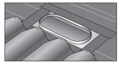
INSPECT existing subflashing has been properly installed in accordance with manufacturer's installation instructions. (See No. 1 in the General Instruction Notes.)
