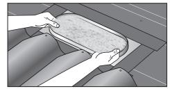
**3. APPLY** pre-cut section of the patented 3-D emberresistant stainless steel vent matrix within the interior lip of the subflashing, fully covering the wire mesh screen. (See No. 2 in the **General Instruction Notes**.)
