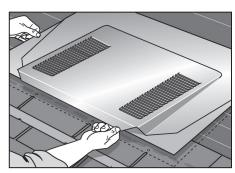
**3. PLACE** vent directly over 11 x 11 inch hole using previously marked outline as a guide.
