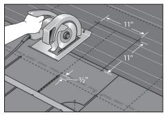
1. MARK & CUT\* Align front of vent 1/2 inch below nail line and mark outline of vent for placement later. Mark outline of 11 x 11 inch hole. With blade set to thickness of sheathing, cut hole in roof deck.
