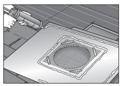
2. SEAL using a sufficient amount of locally-approved sealant (Class A where required by code for flame and ember resistance) around inner and outer flange.
