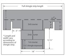
1.TRIM Cut 2 shingle strips to lengths shown for Courses 1 and 2. Using a full length of shingle strip, trim to pattern dimensions shown for Course 3.
