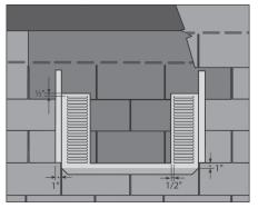
2. BEGINNING WITH COURSE 1 Align and attach to top of vent as shown using locally-approved peel and stick, two-sided tape, or sealant (Class A where required by code for flame and ember resistance). Repeat with courses 2 and 3 to complete shingle-over finish method.
