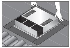
5. FLASH (See No.1 in the General Instruction Notes below.) When using peel and stick or membrane and mastic methods, apply bottom strip first, then sides, and finally the top strip.
