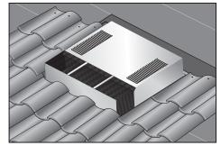
COVER vent flange with roofing material. Secure roofing material using locally-approved roofing nails or screws of sufficient length to penetrate sheathing.
