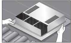
**3. PLACE** vent directly over 14 x 14 inch hole using previously marked outline as a guide.
