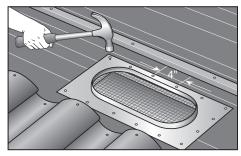
ATTACH subflashing at 4 inch centers, using locallyapproved roofing nails or screws of sufficient length to penetrate the sheathing.
