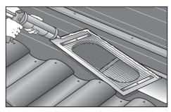
2. SEAL using a sufficient amount of locally-approved sealant (Class A where required by code for flame and ember resistance) around outer flange of primary vent (subflashing).
