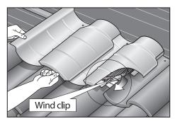
**5. INSTALL** the secondary vent (cover), bending the wind clip tightly under the preceding course of tile, adjusting for head lap.
