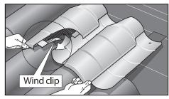
**5. INSTALL** the secondary vent (cover), bending the wind clip tightly under the preceding course of tile, adjusting for head lap.
