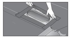
SEAL, ATTACH & FLASH subflashing as shown in Steps 2-4 of the High Profile (S) installation instructions. Apply field tile up to the subflashing, nailing the wire into place.
