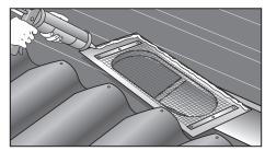
2. SEAL using a sufficient amount of locally-approved sealant (Class A where required by code for ember and flame resistance) around outer flange of primary vent.
