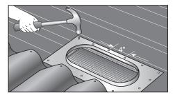
ATTACH subflashing at 4 inch centers, using locallyapproved roofing nails or screws of sufficient length to penetrate the sheathing.
