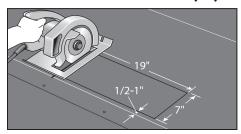
MARK & CUT primary vent (subflashing) opening as shown. Align the bottom of the opening 1/2 to 1 inch above the pan tile layout line as shown. (Note: Set blade to the thickness of the sheathing.)
