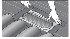
4. FLASH (See No. 1 in the General Instruction Notes below.) When using peel and stick or membrane and mastic methods, apply bottom strip first, then sides, and finally, the top strip.
