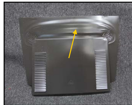
Mill Finish and Pre-Painted Galvanized One-Piece Covers Showing Acceptable Materials Variances
